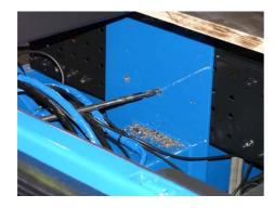
▶ Drill the holes in the console plates.
