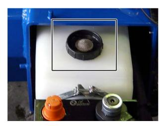
▶ Insert the enclosed air filters.
