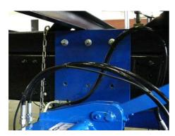
▶ Bolt the console plates to the vehicle chassis. In the process, note the tightening torques in the general installation diagram and in the following table.
