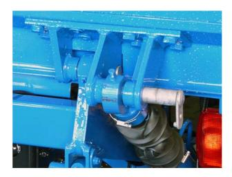
▶ Grease the pin and bolt the tilt cylinder to the platform.
