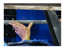
▶ Mark the following holes on the console plate. Observe the general installation diagram and vehicle manufacturer's box body mounting guidelines. Above all, note the number, position and diameter of drill holes.
