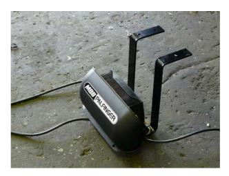
► Fix the control panel holder with screws or weld it in position as per the MBB installation diagram.
